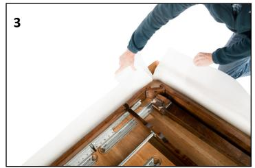
Legs will be installed while table top is in box. Locate legs and clear corner of table where leg is to be installed. Cut foam in corner if more access space is needed.
