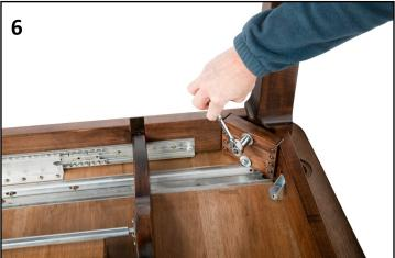
Tighten nuts using rachet with 1/2" socket or 1/2" wrench. Tighten snugly, but there is no need to overtighten. Repeat process for all four legs.
